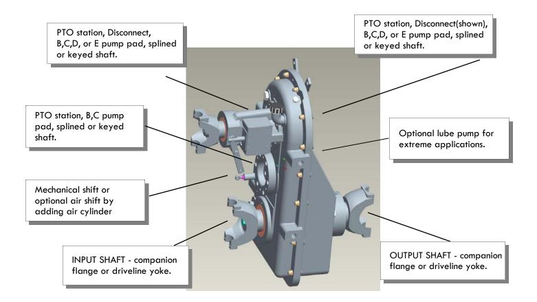
Cotta TR2237 series split shaft PTO's have three PTO stations. Disconnects are available on either top station. Mechanical or optional air actuation for both main shift and disconnect is available. A 1.25 and 1.4 overdrive ratio on the top station is also optional.
