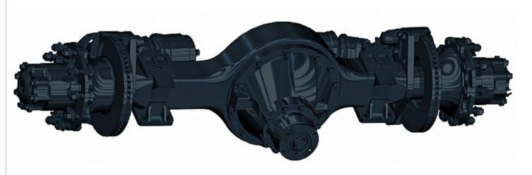
AxleTech's new 7000 Series single reduction rear drive axles are designed for a wide range of off-highway, light to heavy-haul specialty trucks. Our 7000 Series single reduction drive axles are available in single and tandem configurations with axle weight ratings up to 30,000 lb (13.6 T) and 72,000 lb (32.6 T) respectively. Axles are available with drum or disc brake options, an overall axle ratio range of 2.85 to 6.83, and multiple track widths to meet vehicle specifications.
